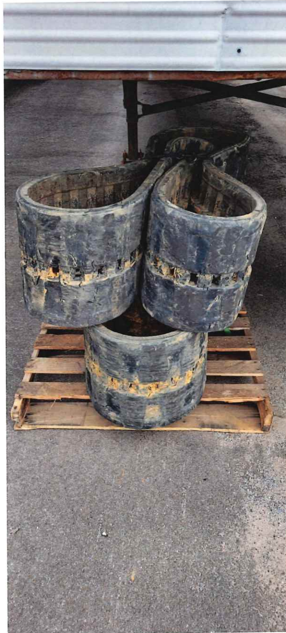
Worn out tracks for Kubota track hoe.
