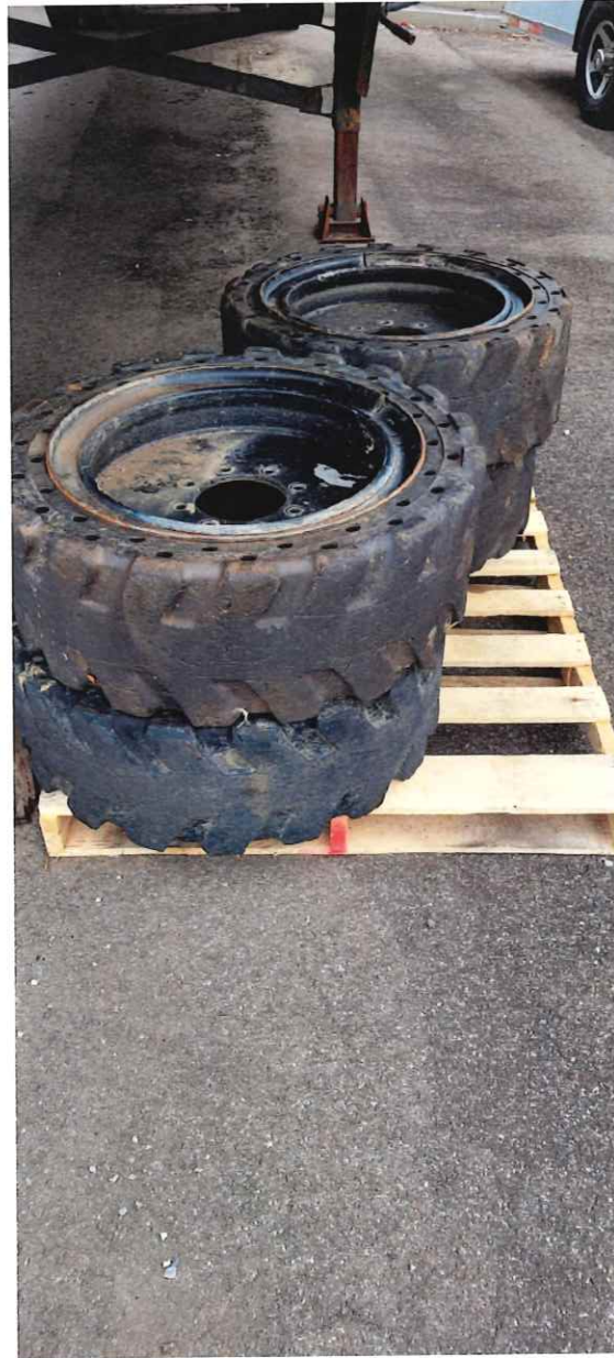
Worn out bobcat solid tires and rims.
